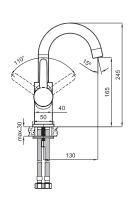
Comfort Length: 130 mm Comfort Height: 165 mm 35 mm ceramic cartridge 360° swivel spout Honeycomb aerator
